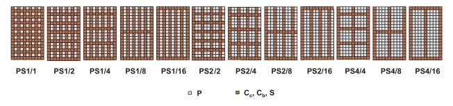
**Figure 3** Schematic diagram of open-grid structures formed in the woven fabrics (dark squares: metal composite yarns: light squares: PET yarns).
