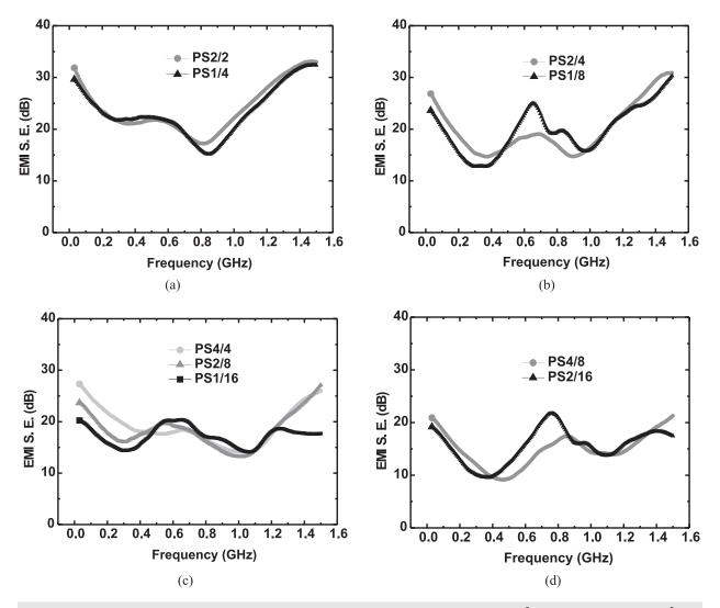
**Figure 10** Effect of shape factor on the EM shielding effectiveness (a) openness  $\approx 0.63 \text{ mm}^2$ ; (b) openness  $\approx 1.26 \text{ mm}^2$ ; (c) openness  $\approx 2.53 \text{ mm}^2$ ; and (d) openness  $\approx 5.06 \text{ mm}^2$ .
