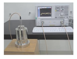
Figure 4 Set up of EMSE testing apparatus.
