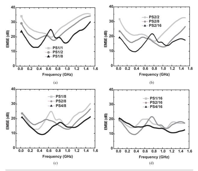
**Figure 8** Effect of grid openness on EM shielding effectiveness (grid size increased in the weft or warp direction). Fabrics with the same warp opening ( $d_{WA}$ ): (a)  $d_{WA} \approx 0.40$  mm and (b)  $d_{WA} \approx 0.79$  mm; fabrics with the same weft opening ( $d_{WE}$ ): (c)  $d_{WE} \approx 3.18$  mm and (d)  $d_{WE} \approx 6.35$  mm.
